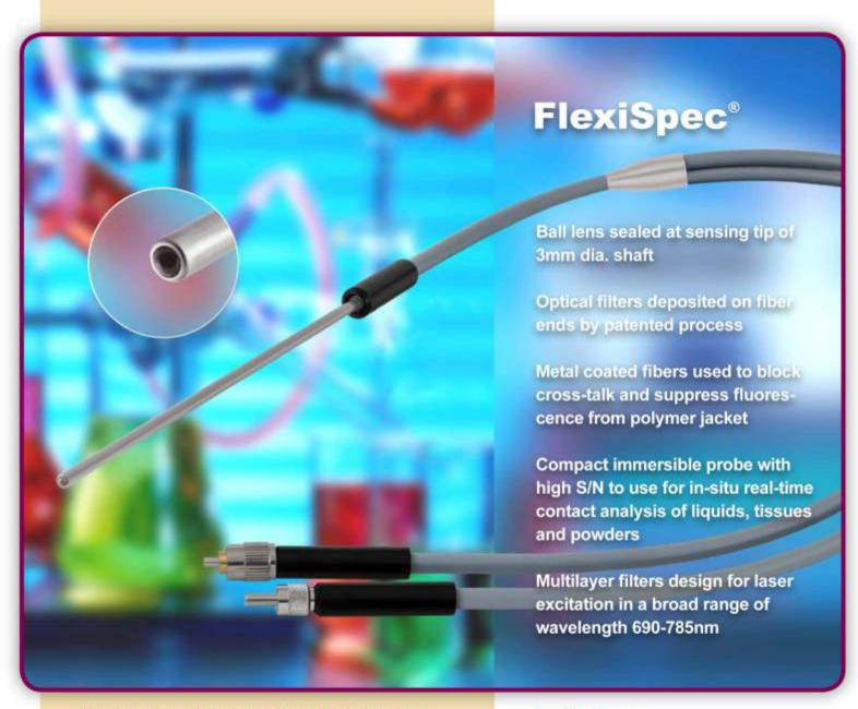
Ball-lens Raman fiber-optic probe is a new addition to art photonics' FlexiSpec® product line.
